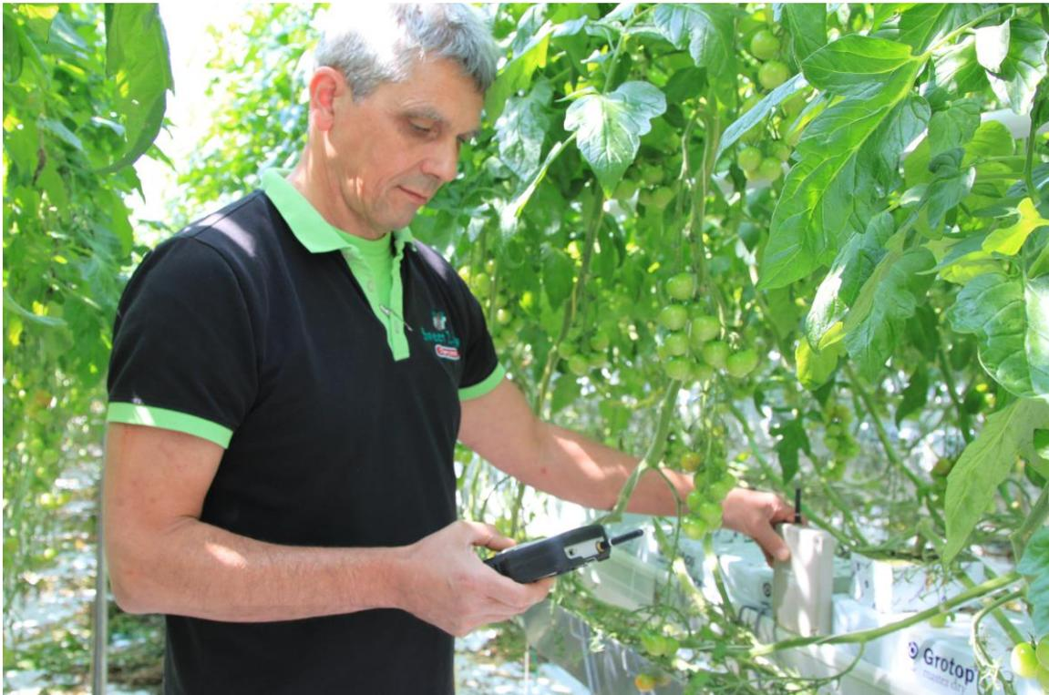
Besides the six fixed wireless sensors Janssen also uses the flexible GroSens handheld for additional measurements.
