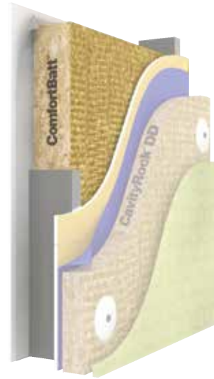
In the ROXUL BEDR™ Wall system, COMFORTBATT Steel Stud insulation allows builders to achieve a thermal value of R-24 and offers superior acoustical performance in comparison to traditional steel stud wall cavities.
