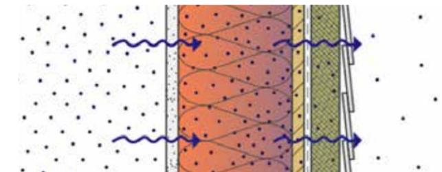
Figure 8: Vertical Section through Insulated 2x6 Wall with Vapour Permeable Exterior Rigid Insulation
