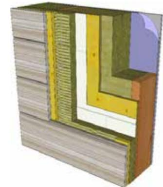
Figure 7: Split insulated wall assembly with mineral wool insulation installed over a 2x6 insulated wood-frame wall
