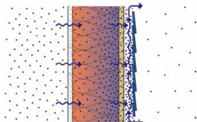
Figure 6: Vertical Section through Insulated 2x6 Wall with Ventilated Impermeable Cladding
