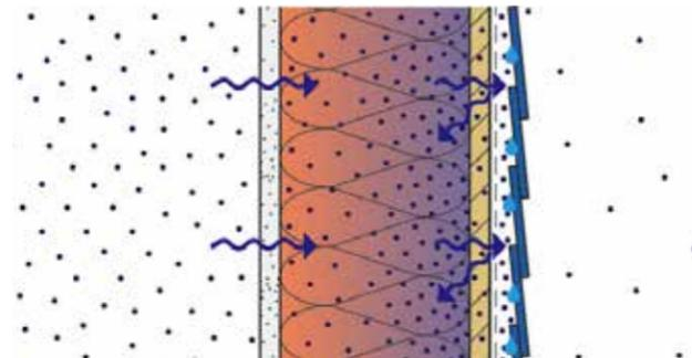
Figure 5: Vertical Section through Insulated 2x6 Wall with Vapour Impermeable Cladding
