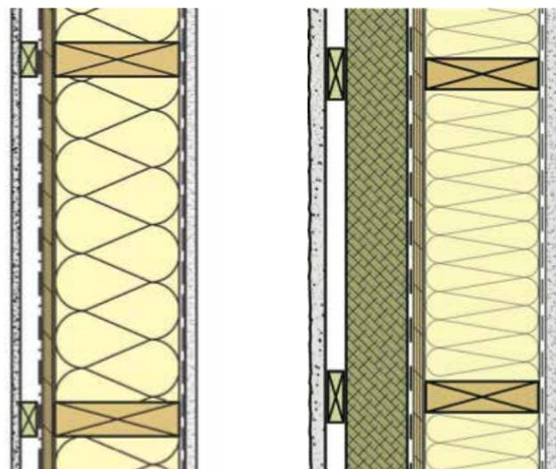
Traditional stud insulated wall assembly (left) vs an improved R-value split-insulated (insulation outside the sheathing as well as in the stud space) wall assembly (right) – The selection of insulation type and vapour control strategy is different for each wall.
