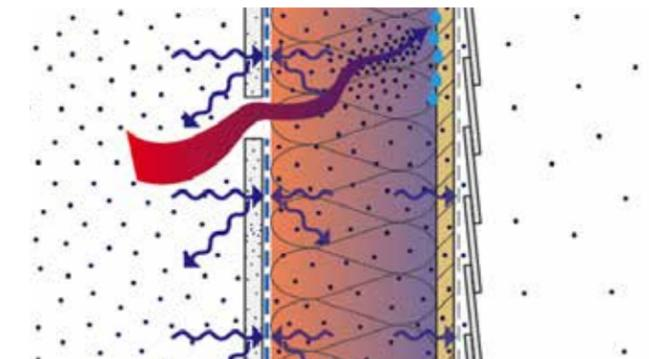
Figure 3: Vertical Section through Insulated 2x6 Wall with Air Leakage Condensation
