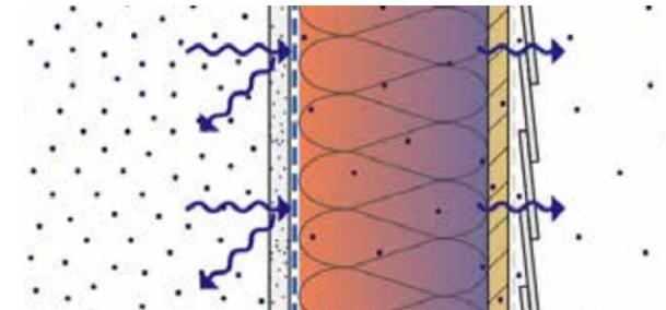
Figure 2: Vertical Section through Insulated 2x6 Wall with Interior Vapour Control (Polyethylene)
