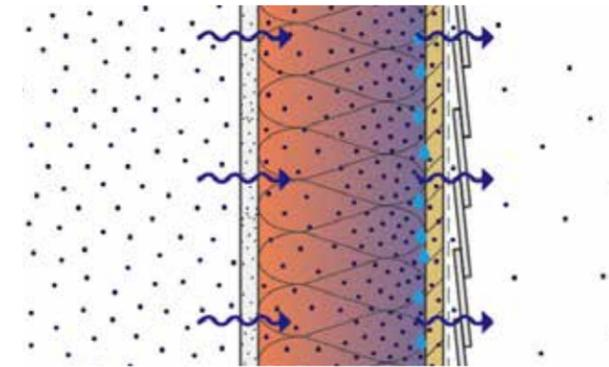
Figure 1: Vertical Section through Insulated 2x6 Wall without Interior Vapour Control
